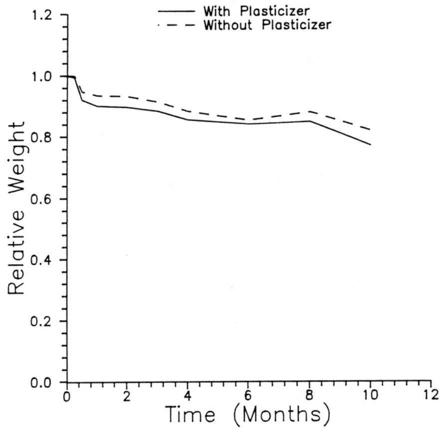
**Figure 1.** Weight Loss of Filter Tips with and without plasticizer.
